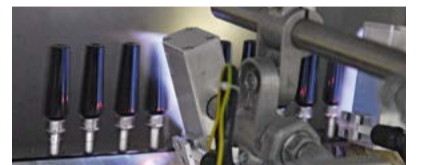
Activation of the surface via flame treatment
