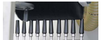
Removing dust of the parts in a brushing station
