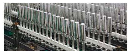
Up to 18,000 parts per hour are coated on the Sprimag machine
