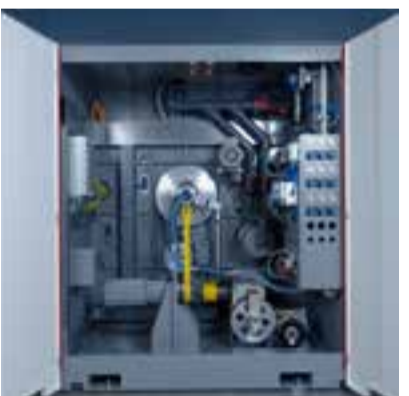
Cleared up components and free access for maintenance work: Moving the exhaust unit creates space and cleanliness.
