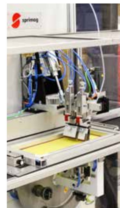
The two squeegees can be fully adapted to the different piston types without a tool.
