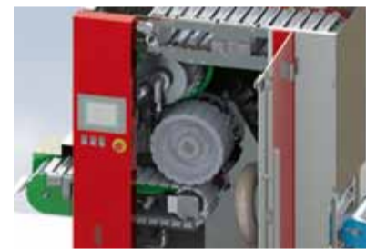
The belt transportation system works without format parts.
