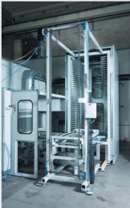
The control system evaluates the signals from the sensors and starts spraying using the newly developed S-7 spray gun from Sprimag. The control system also operates the oscillating motion of the spray gun with help from linear sensors stop spraying after the plate passes. The spray stroke speed of the spray axis, and spray cycles can individually be programmed into the control system.
