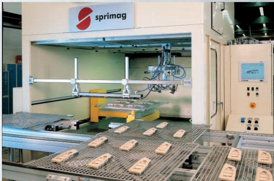
Spray Station with flexible Pallet Conveying System
