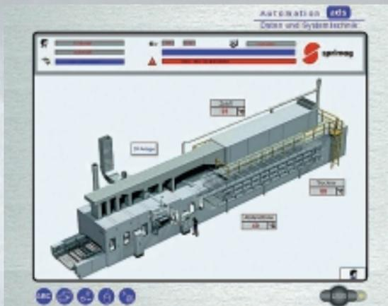
In case of a malfunction alarm, a warning symbol is shown in the display. When selecting the symbol, the operator enters into a menu of malfunctions. In this menu, the kind of malfunction is described by a short text, and the place where the malfunction occurred is shown. For trouble shooting a corresponding list of recommendations can also be displayed.
