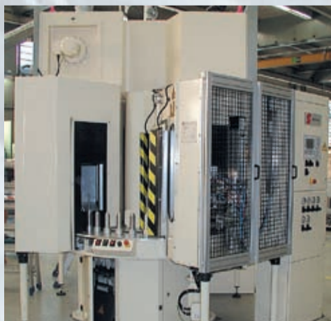
Sprimag Round Table Coating Machine for coating of parts with a rubber-to-metal bonder Sprimag Rundautomat zum Beschichten von Gummi-Metall-Bindemittelteilen
