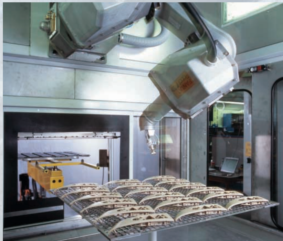
Coating by Robot / Roboterlackierung
