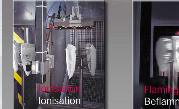
SPRIMAG has planned and realized a universal "spindle lacquering unit" for coating metal and plastic parts for a job shop.
