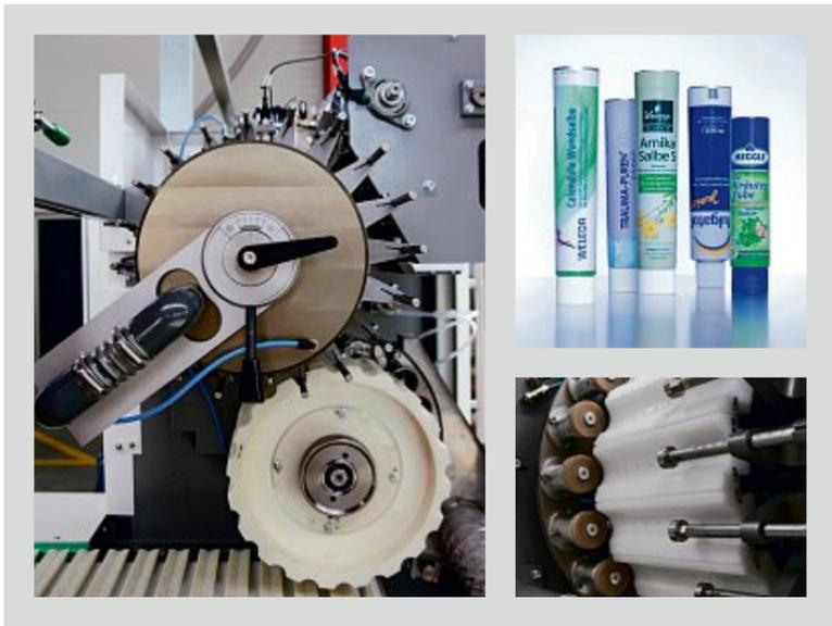
20 testing heads test up to 200 aluminum tubes per minute for leaks
