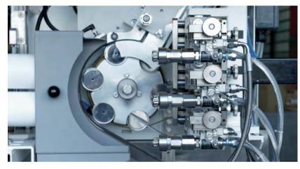
For certain applications, the HIL-34 can also be equipped with three instead of two spray guns, thereby lacquer can be saved.
