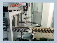
Transfer station on discs with object identification for the production in mixed operation
