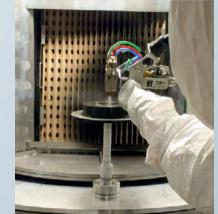
The coating robot is equipped with two Sprimag spray guns, thus different requirements regarding the coating layer can be met
