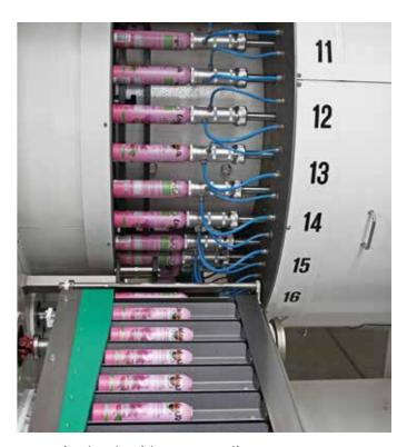
30 testing heads with proven sealing system guarantee a sufficiently long cycle time and precision
