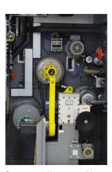
Compact servo drive concept with seperate servo drives for stroke and transport movement and good accessibility for maintenance
