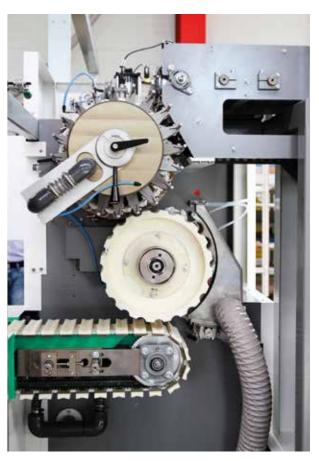
Drum concept for precise positioning of the aluminum tubes
