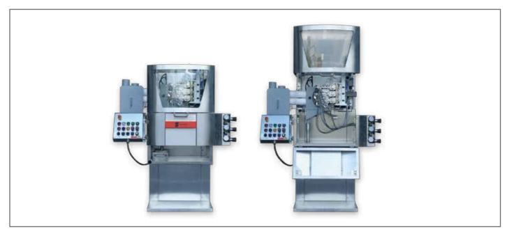
Optimized accessibility due to automatable cover panel lift
