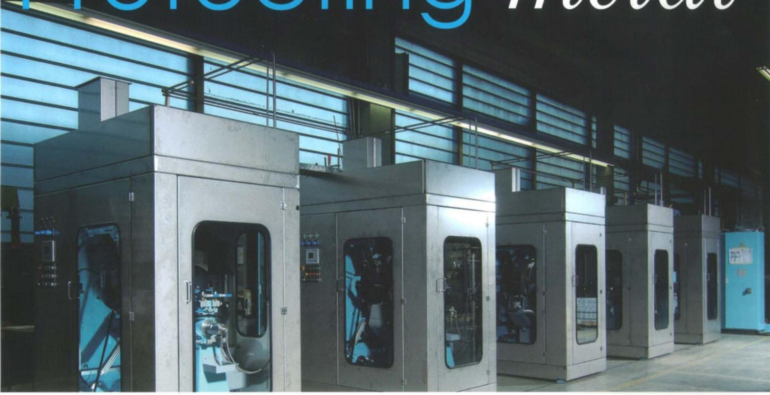
The modules of Sprimag's HIL-15 coating machine can handle 900 cans per minute each
