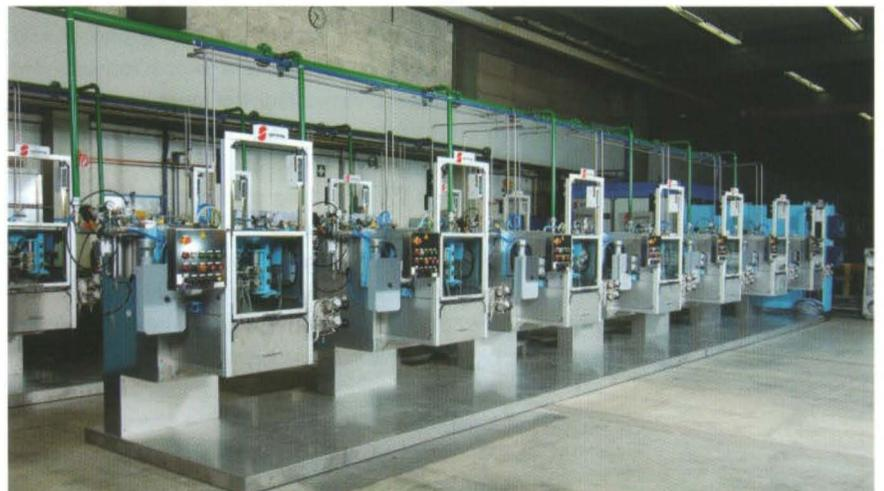
*Sprimag's HIL-34 internal coating machine is used on beverage cans*
