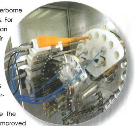
*Sprimag's HIL-70 internal coating with powder*
